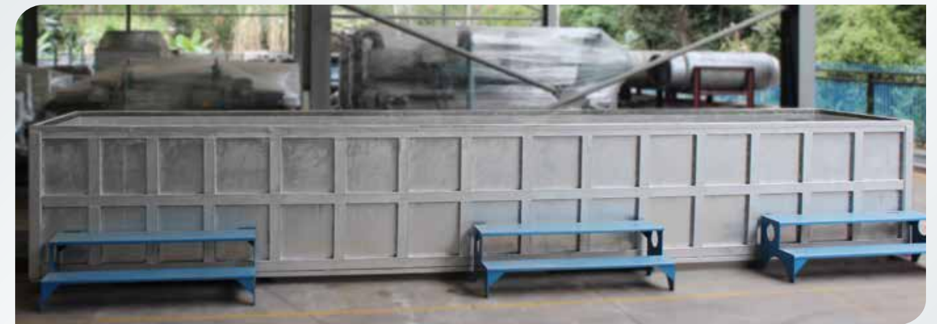
◆ Large Pressure Test Tank
